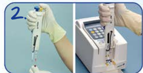
Draw the sample and reference solution with the twin-pipette. Set pipette and apply sample to E-plate
