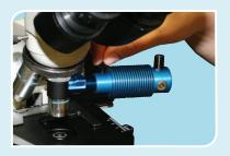
Tighten thumb screw until light source is held securely.
