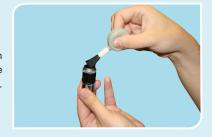
Use a sheet of lens paper to wipe oil residue off of the objective after every use.
