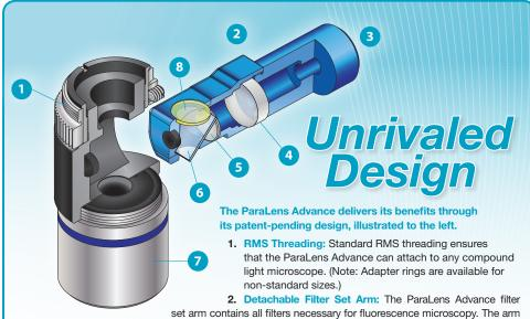
slides into the main body of the ParaLens Advance and is held into place through a pair of powerful magnets.
