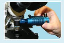
Slide LED light source onto filter set arm.
